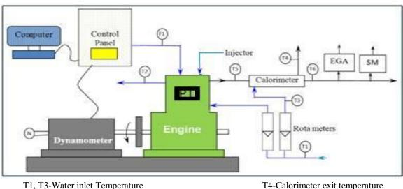
11, 13- Water inlet Temperature14-Calorimeter exit temperaT2-Engine water jacket outletT6- EGT after CalorimeterPT- Pressure transducerEGA-Exhaust gas analyzerN-RPM encoderSM-Smoke Meter
