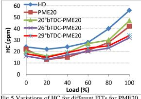
Fig.5 Variations of HC for different FITs for PME20 *4.5 NOx*
