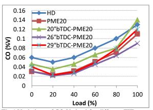
Fig.4 Variations of CO Vs load for different FITs whereas it was 0.09%v for HD fuel normal operation, at 80% of full load.
