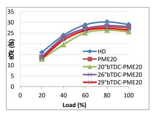
Fig.2 Variation of BTE for different ITs for PME20
