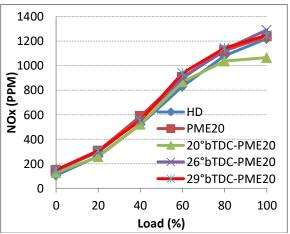
Fig.6 Variation of NOx for different FITs for PME20
