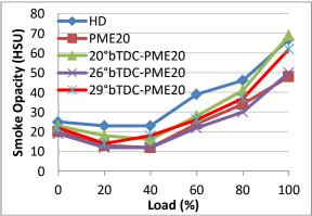
Fig.7 Variations of Smoke for different FITs for PME20 fuel
