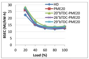
Fig.3 Variation of BSEC with load for different FITs for PME20 fuel
